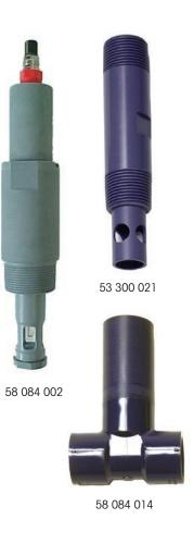
METTLER TOLEDO Thornton housings provide a fixed NPT or solvent weld process connection. For easy access to the electrode for cleaning, calibration or replacement, they have internal O-ring seals with hand-tightened mounting nut. The compact METTLER TOLEDO electrode design includes measuring, reference and fast-responding temperature compensator functions so only a single process connection is ever needed.
