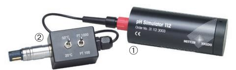
pH Analog Verification Kits: Combining the pH simulator 112 ① with the VP simulator ② both pH and Temperature signals can be simulated to check the automatic temperature compensation capability of the transmitter.
