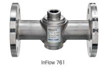
InFlow 76X flow-through housings from METTLER TOLEDO are designed to enable safe and reliable mounting of the InTrac and InFit series sensor housings directly into the process or in a bypass (pipe). These rugged flow-through housings are specially suited to the requirements of the process industry and can be easily and safely installed, allowing reliable measurement procedures.
