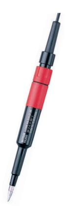
Puncture pH electrodes are specially designed for quick, accurate pH measurement in meat, sausage, cheese, and fruit. The rugged needle-shaped sensing membrane penetrates directly into the medium, without requiring time-consuming sample preparation. The solid polymer reference system eliminates clogging by fats and proteins using an open junction design. The non-refillable reference electrolyte reduces maintenance to a minimum.
