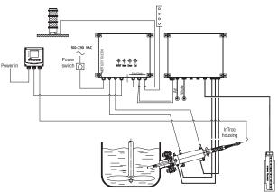
Schematic of a typical EasyClean custom installation
