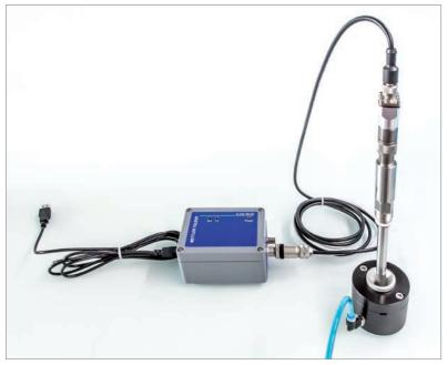
**iLink Multi** is a universal device for connecting digital ISM sensors (1-wire; RS 485) to a PC/laptop running iSense software. When calibrating an optical DO sensor with the iLink Multi, calibration parameters are captured automatically using the built-in, physical parameter sensors.
