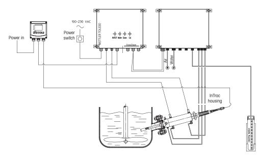
Schematic of a typical EasyClean 200e installation
