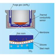
Fig 1: TC sensor design-complete avoidance of moving parts
