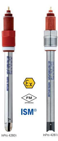
The InPro 4260 (i)/InPro 4281 i is a combined pH electrode and temperature sensor family designed for highly demanding chemical applications. InPro 4260 (i)/InPro 4281 i electrodes feature Xerolyt® Extra polymer reference electrolyte for precise pH measurement and longer lifetime, even under the most difficult industrial environments. Also available with Intelligent Sensor Management (ISM) for Plug and Measure and advanced diagnostics.
