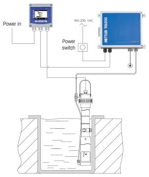
Schematic of a typical EasyClean 100 installation
