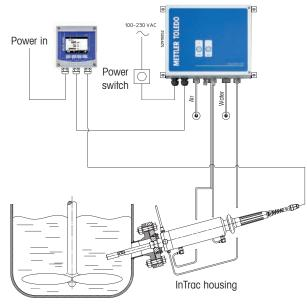
Schematic of a typical EasyClean 150 installation
