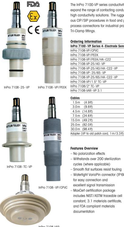
The InPro 7100-VP series conductivity sensors utilize 4-electrode technology to expand the range of contacting conductivity for the measurement of medium to high conductivity solutions. The rugged sensor design withstands the most rigorous CIP/SIP procedures in food and pharmaceutical industries. Series includes process connections for industrial processing as well as hygienic 25 mm port and Tri-Clamp fittings.
