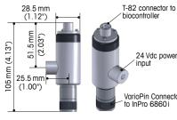
24 Vdc power VarioPin Connector to InPro 6860 i
