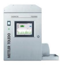
METTLER TOLEDO Thornton's 7000RMS<sup>™</sup> (Real-time Microbial System) is an at-line analyzer for real-time measurement of microbial contamination (bioburden) in Pharmaceutical Waters. Advanced, laser-induced fluorescence and Mie scatter-ing measurement technology provides immediate detection and quantification of microorganisms. The compact analyzer overcomes limitations of growth-based technologies that are dependent on incubation conditions, growth media, reagents and time.
